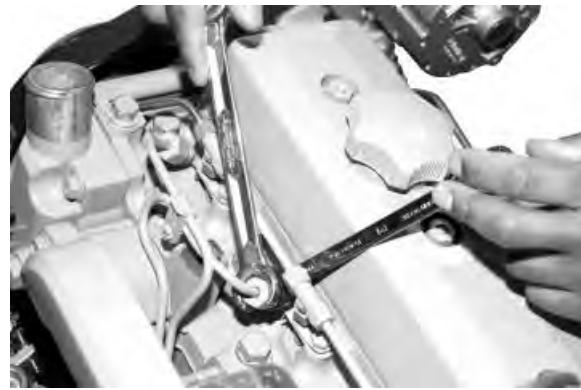
Bleed Fuel System at Fuel Injection Nozzles
