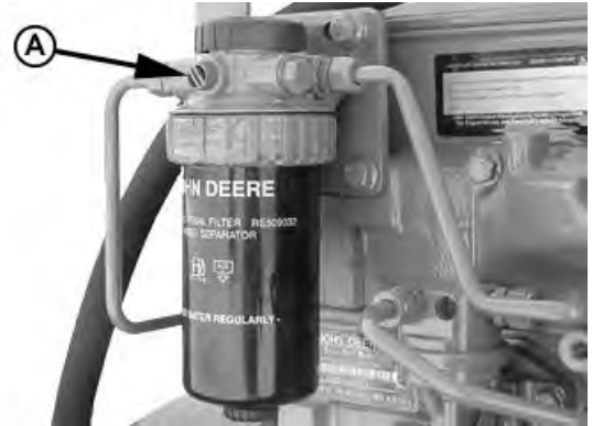
Final Fuel Filter Bleed Screw
